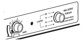
NOTE: Attempting to force the timer control to CONSTANT ON by turning the timer knob clockwise (past the 12 hour mark) will cause damage to your unit.
