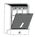
5. Replace the Filter Assembly, inserting the bottom of the Filter Assembly first.
