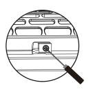
4. Use the included screwdriver to unscrew the Filter Assembly.
