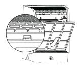
1. Install the Filter Assembly by inserting at the bottom.
