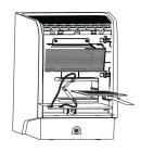
Gently insert the Purification Plate between the guides (inside the cage) until it stops.
