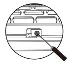
4. Use the included screwdriver to screw in the Filter Assembly.
