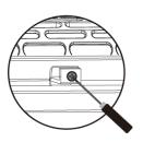
2. Use the included screwdriver to secure the Filter Assembly.
