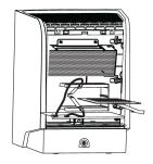
To remove the Purification Plate, grasp edge of plate in the center and gently pull out.
